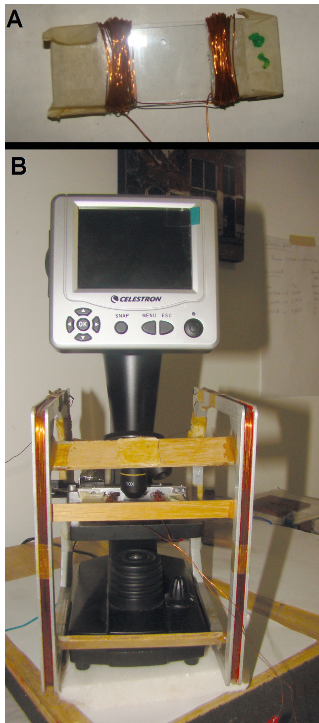
Fig. 1. A — Glass microscope slide with a pair of coils to generate the magnetic field B_{DC} . The optical plane is on the glass surface and corresponds to the X — Z plane while the positive Y-axis points up. B — Experimental set-up. The digital microscope Celestron is inside a pair of coils used for the generation of the magnetic field B_{AC} . The microscope slide of figure A is fixed on the microscope stage; observe that both coil axes are parallel.
