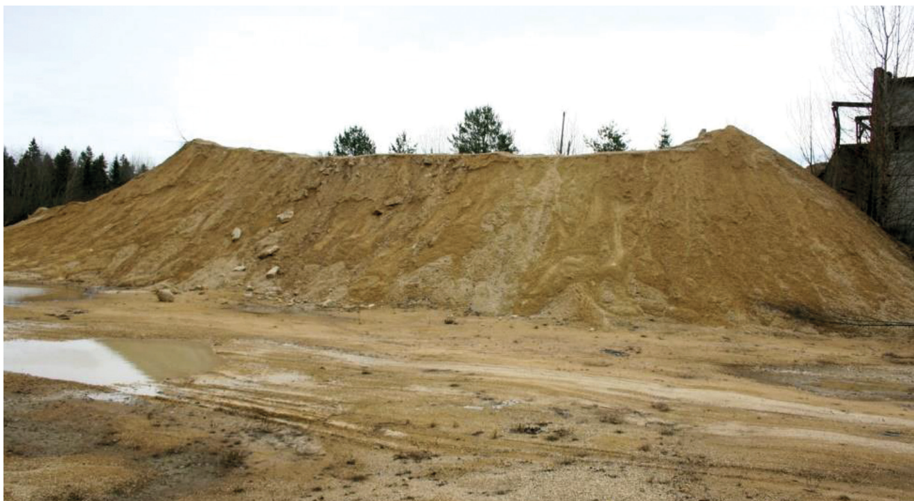
Fig. 1. Dumps of dolomite dropouts from stone processing factory, in St Petersburg region, Russia.
